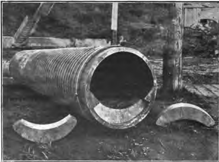
FIG. 350.—THE HOPKIRK WOOD PIPE, FOR CARRYING GRITTY MATERIAL, THE WEAR BEING UPON THE END GRAIN OF THE WOOD.
