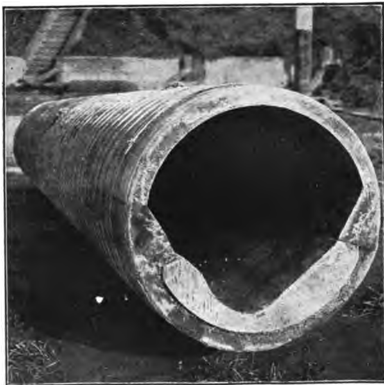
FIG. 351.—THE HOPKIRK PIPE, AFTER SIX AND ONE HALF MONTHS WEAR ON 20% GRADE, IN SEATTLE.
